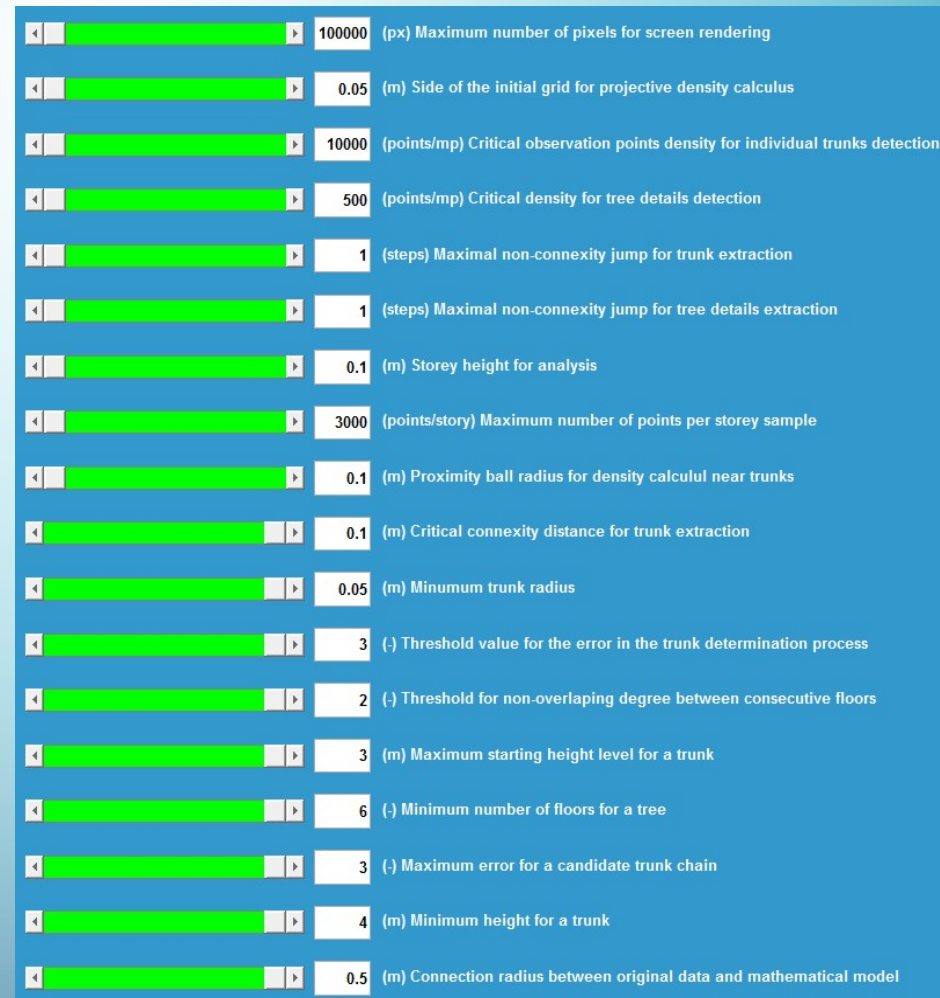
Figure 4. Main control panel, with 18 of the most important parameters of the system. The user must be well trained for a good usage of the panel. All the parameters are kept inside predefined intervals of variation.
