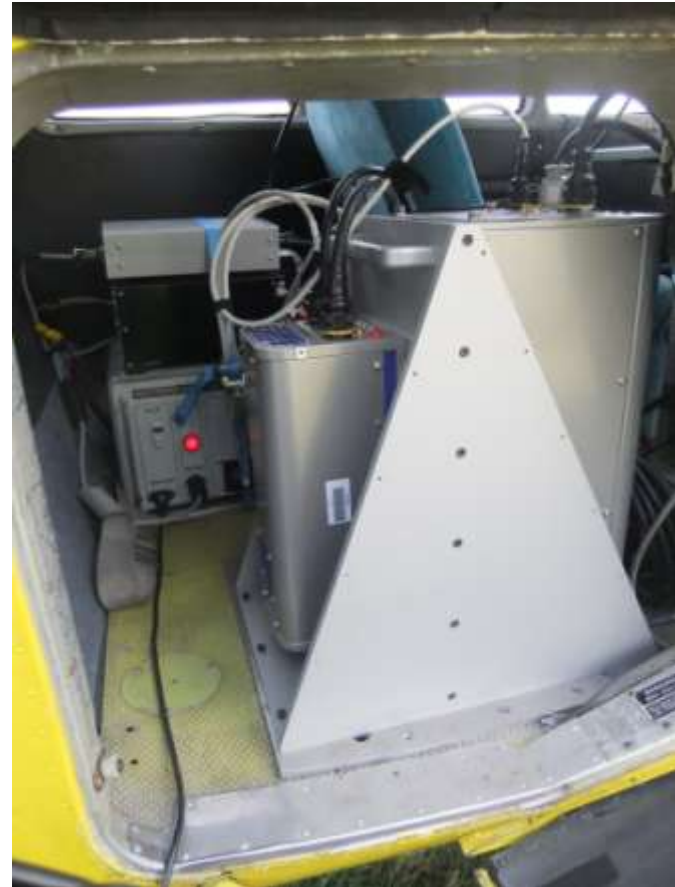
The sensor was mounted to a Piper Aztec aircraft.
