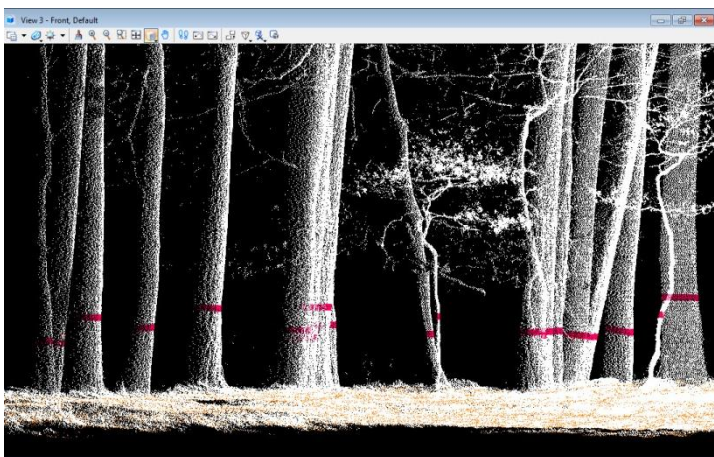
Classified point cloud (red slices; BHD 1.28-1.32 cm above ground)
