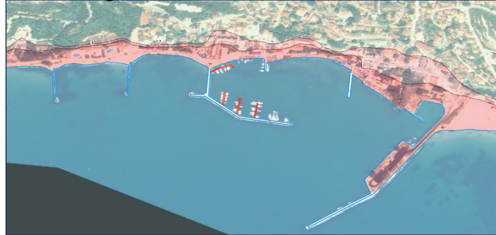
The 3 rd and 7 th -meter contour lines were generated and the coastal infrastructure and installations, potentially endangered by high waves were identified.
